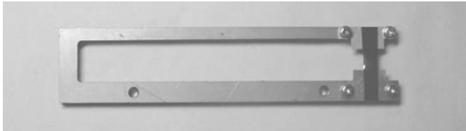
Fig. 6. TR target containing one C layer with a thickness d = 265\text{--}310 nm, onto one collodion layer with a thickness 270–300 nm.
