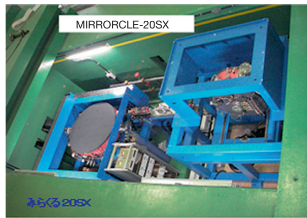
Figure 2 MIRRORCLE-20SX tabletop synchrotron. This machine is installed in a 3 \times 5 \text{ m}^2 wide and 2 m high shielding room. An EUV and soft x-ray beam is extracted downward from the storage ring and can be delivered any place requested.
